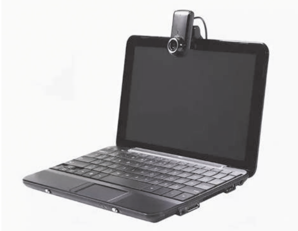
Fig. 1. Laptop vibration is transmitted to the camera
